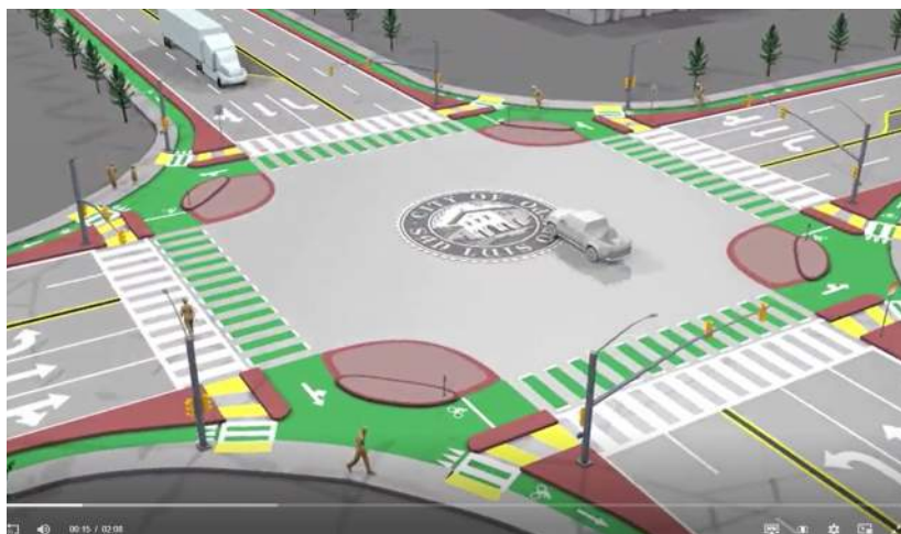
Figure 45: Protected Intersection Graphic from the City of San Luis Obispo
